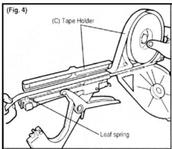
It might happen that the tape catch will not catch the tape end when you press the handle. (This is not trouble with the tapener.) If this happens, press the handle harder several more times, and the tape catch will return to its normal position. (NOTE: This should be done only when the tape catch does not catch the tape end.)
