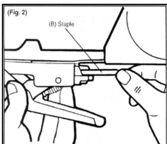
Pick up the staples (B) with right hand and load them into the magazine unit with the staples legs pointing downward; then set them in the pusher unit. (Fig 2)
